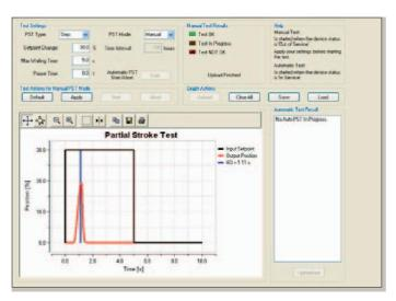
D3 and ValveSight allows "Parial Stroke Tests" to be performed and recorded.
